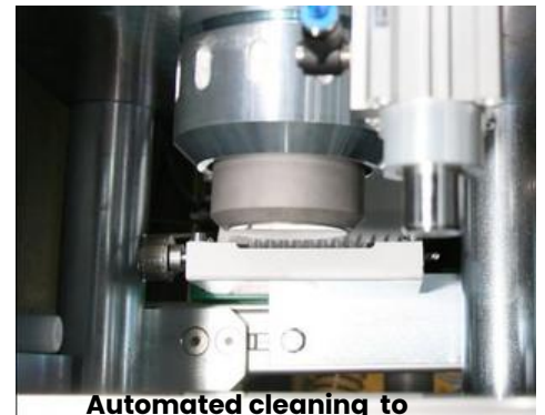
Automated cleaning to prevent contamination
